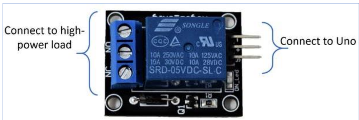
(Figure: 35 Relay Connections)
